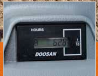
Hour meter (from ground level)
